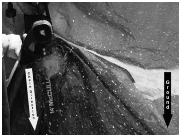
FIG. 9—A vertically oriented electric chainsaw cutting a log illustrating the lateral discharge of sawdust.
