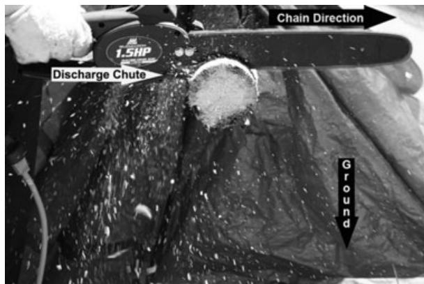
FIG. 8—A horizontally oriented electric chainsaw cutting a log illustrating the downward discharge of sawdust. The discharge chute and chain direction are noted.
