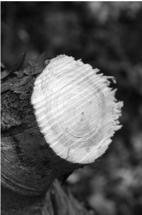
FIG. 11—Cut surface of a piece of wood cut with a chainsaw.
