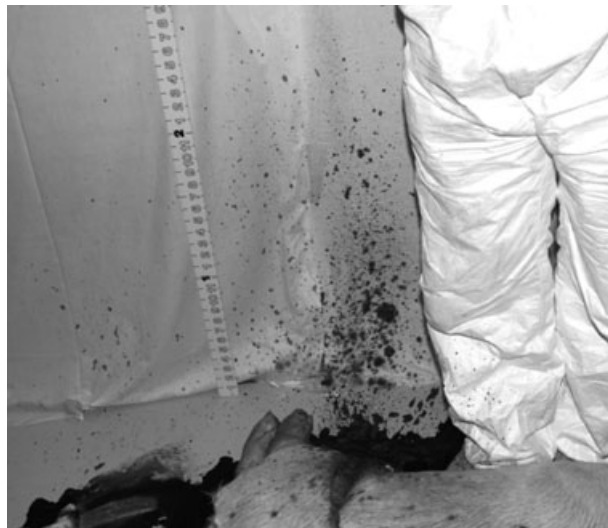
FIG. 7—More extensive spatter on the back adjacent wall when a freshly killed pig was dismembered with a more vertically oriented chainsaw, compare with Fig. 5.
